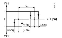
Cooling mode (chilled water) (DIP switch no. 4: OFF)
